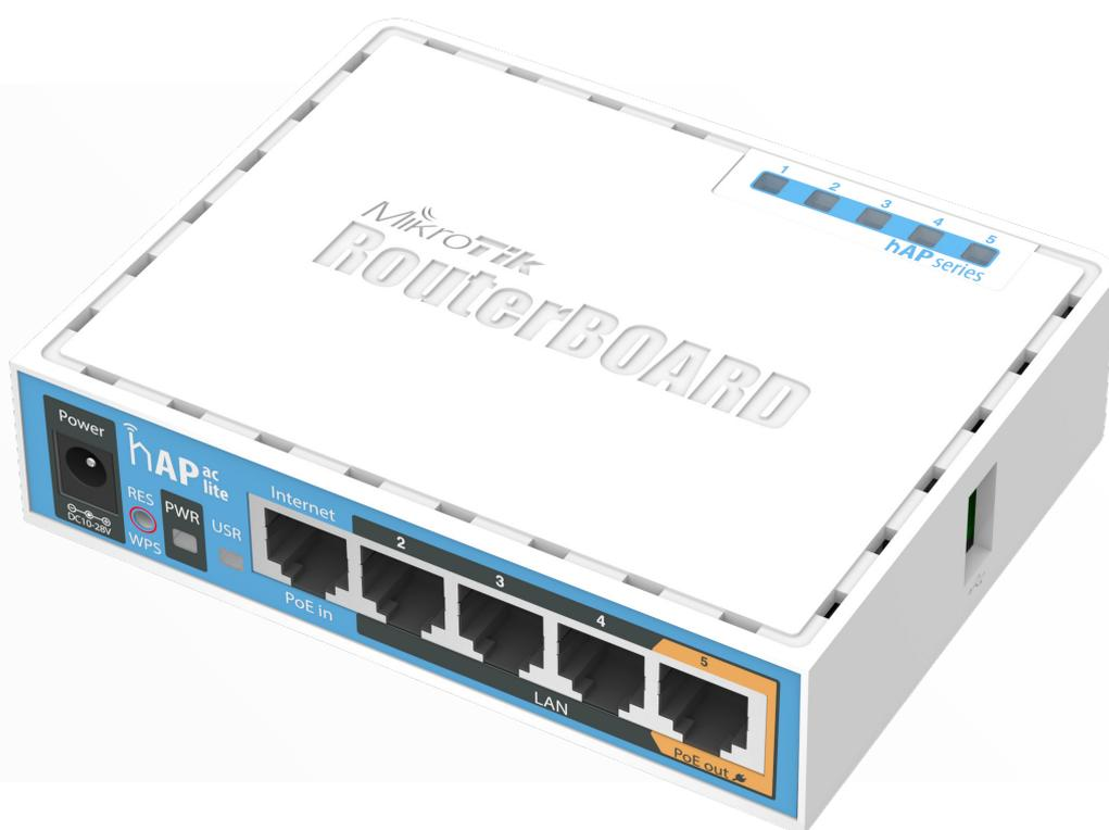
The hAP ac lite can be powered from the power jack or with passive PoE from a PoE injector. The power adapter is included. Unit provides PoE output function for port 5 - it can power other PoE capable devices with the same voltage as applied to the unit. Maximum load on the port is 500mA.
