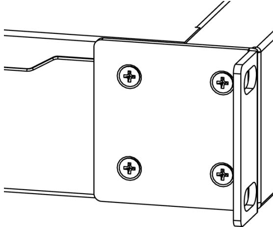
2. Place the device in rackmount enclosure and align with the holes so that the device fits conveniently.
