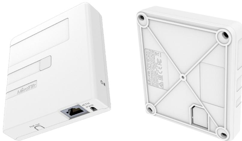
GPEN11 can be mounted inside customer premises, next to the wireless router which provides connectivity to the users. The GPEN11 itself will then power the ISP router, whether it is an outdoor wireless unit mounted on the roof or a network switch somewhere in the building. The GPEN unit can be securely attached to a wall or the communications cabinet. The Ethernet cable can be routed either directly through its bottom cable opening or into the wall, as preferred.
