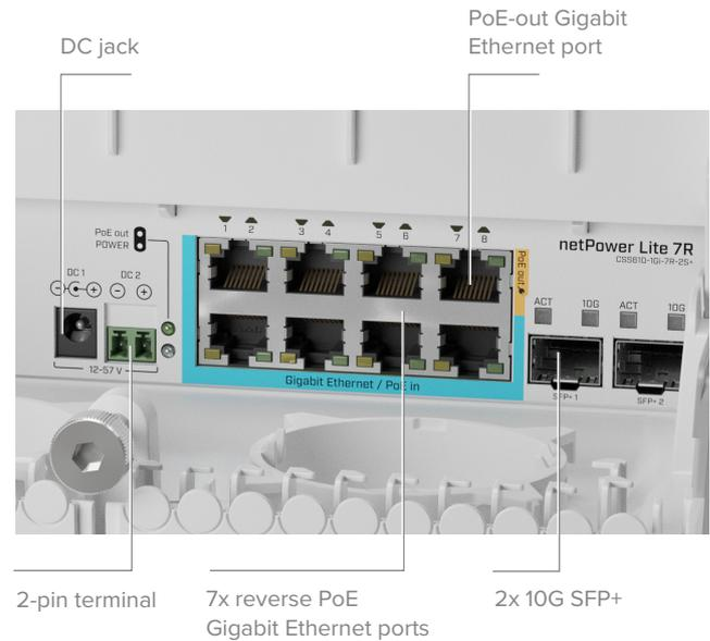
This version of the innovative netPower switches features 8 PoE Gigabit Ethernet ports and 2 SFP+ ports for 10G fiber connectivity.
